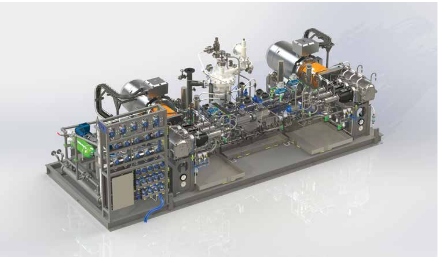
Figure 3: Shipboard high pressure fuel supply system
