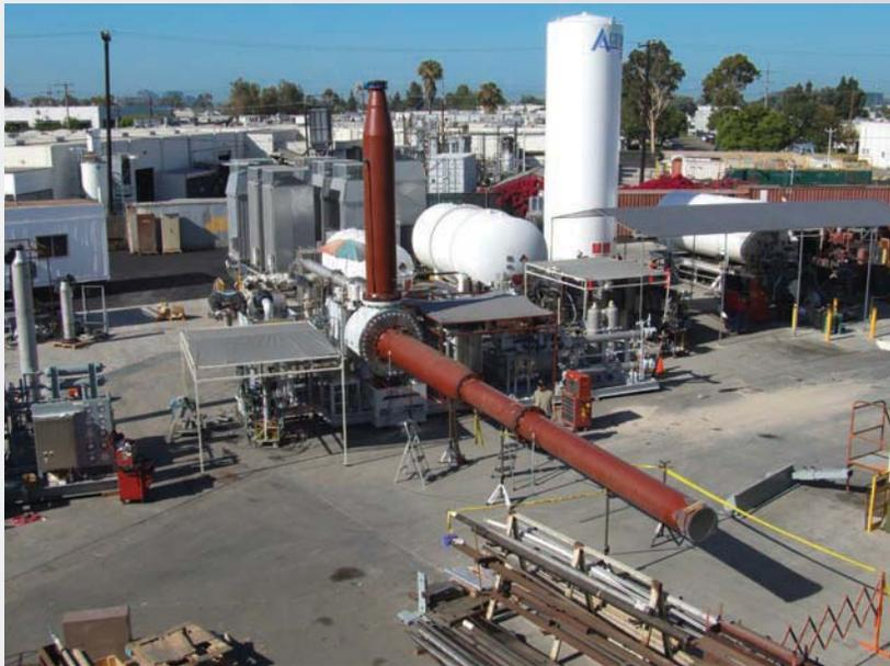
Shipped to the Pacific Rim late last year, ACD's largest set of turboexpanders will be commissioned in 2009. Both the TC-12000 and TC-9000 deliver almost 3300 hp of refrigeration for the plant process. Both were cryogenically tested before shipping, and proved to exceed the guaranteed customer requirements. These units were designed to
