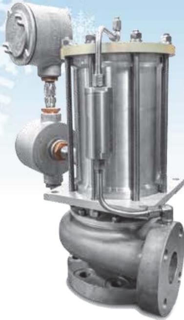
All cryogenic pumps face two operational challenges. First is running two phase flow, that is supplying the pump with liquid close to its boiling point, and second is insufficient initial pump cool-down. Either case will lead to cavitation, resulting in pump damage and reduced life.
