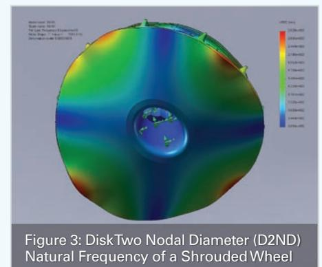
Figure 3: Disk Two Nodal Diameter (D2ND) Natural Frequency of a Shrouded Wheel
