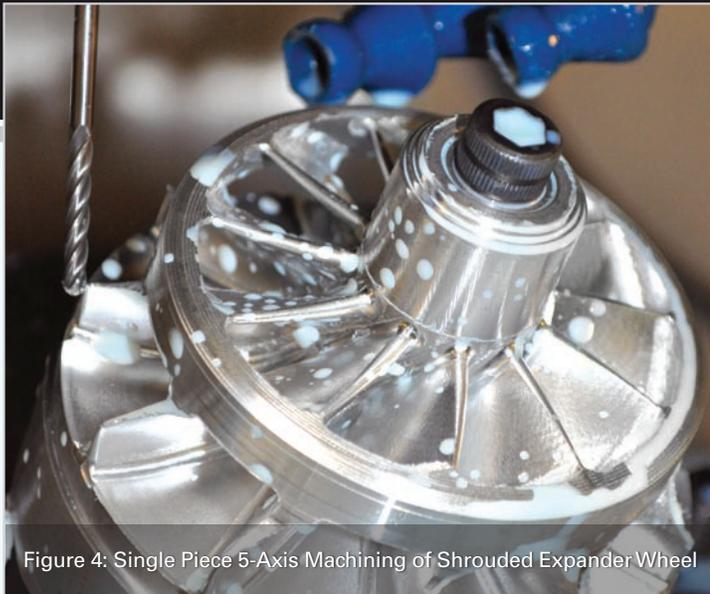
Figure 4: Single Piece 5-Axis Machining of Shrouded Expander Wheel
