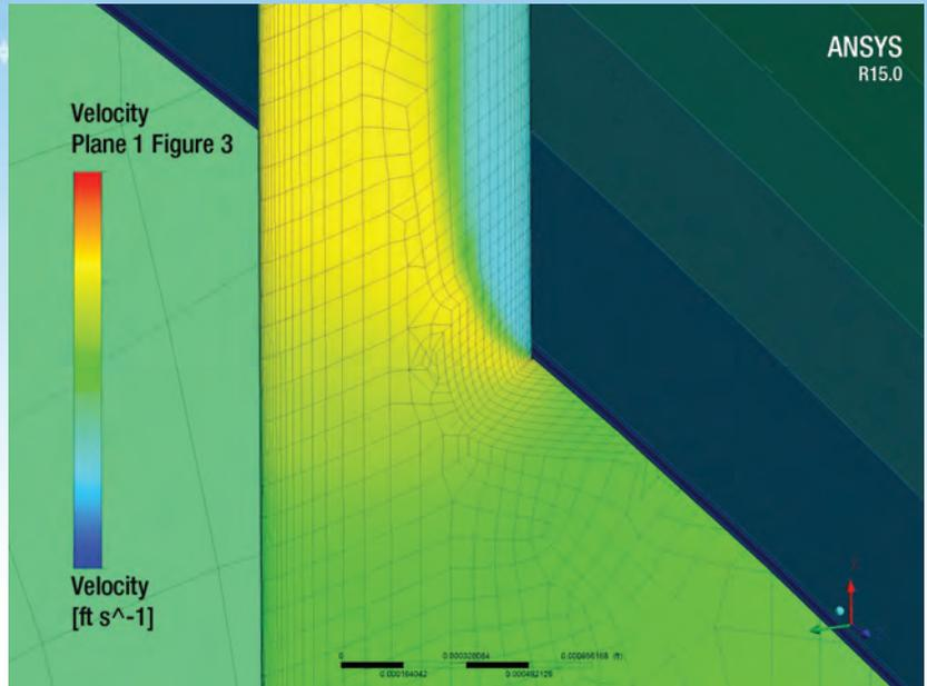
Figure 2: Boundary Layer at Impeller Laby Seal Entrance
