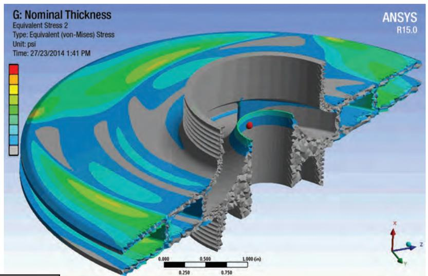
Figure 3: FSI Stresses - Combined Centrifugal and Pressure Load
